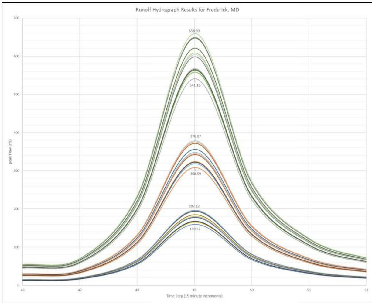
*Figure 9. Ensemble of Hydrograph Results from Scenario Modeling*
